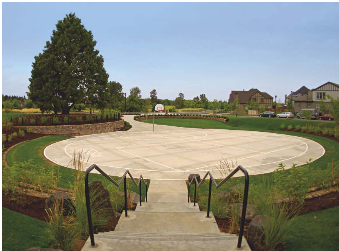
MANY SPACES do double duty at Villebois, such as this basketball court. After a heavy rainfall, it becomes a retention pond.
